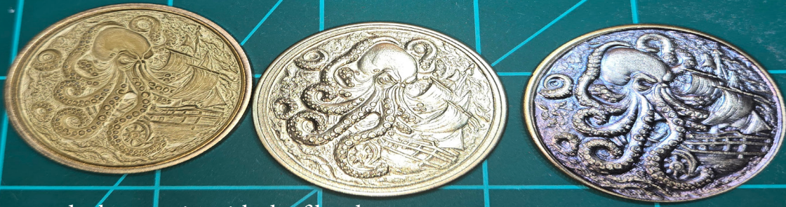
Tony Cardiel carved a brass coin with the fiber laser.
