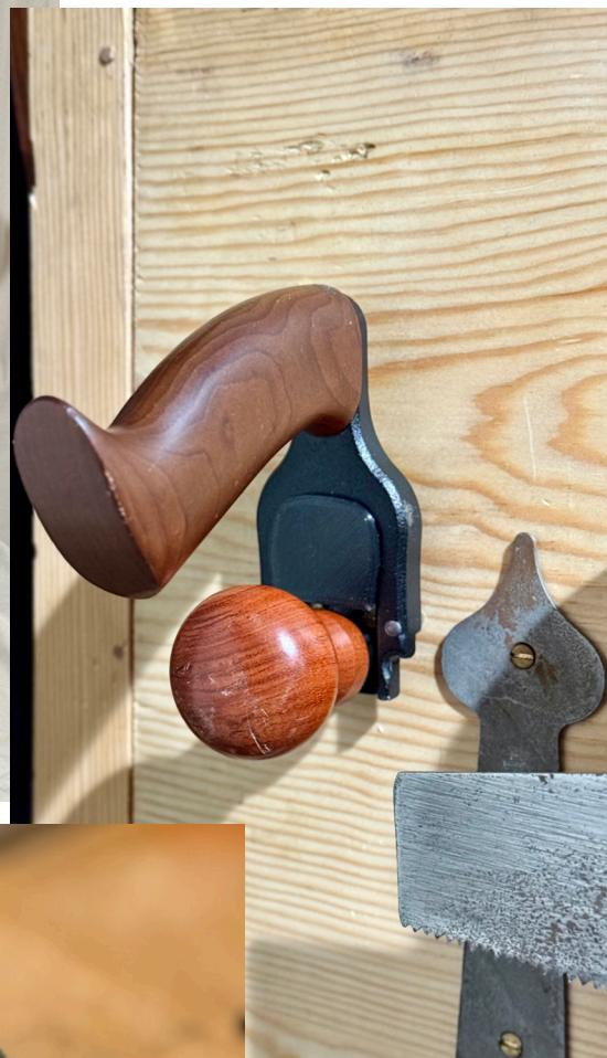
A 3D printed a chamfer guide for my Lee Valley block plane that I used to relieve the edges on the teak bench handles.
